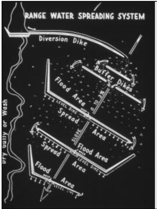
Figure 15a. Water spreading should be considered in arid regions with thunderstorm type rainfall. Flood waters are diverted from the stream channel and spread across the flood plain.
